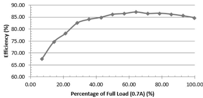
Figure 16. Efficiency vs. Percent Load for Discharging Flyback
