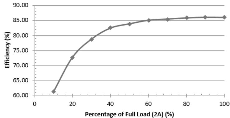
Figure 14. Efficiency vs. Percent Load for Charging Flyback
