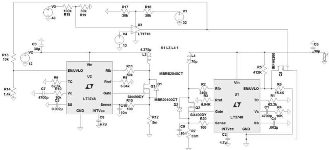
Figure 11. Full Bi-directional DC-DC Converter LT Spice Design
