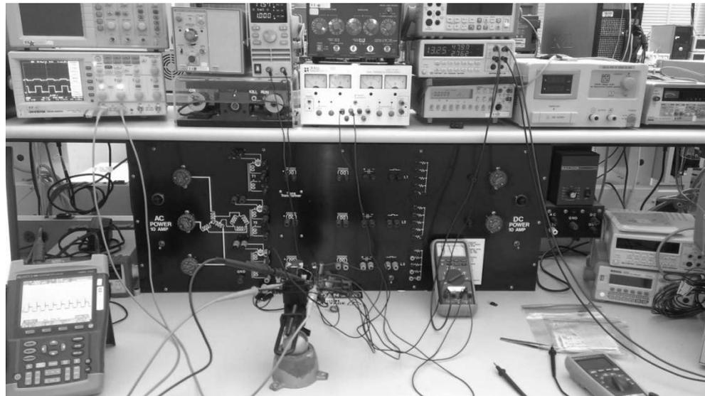
Figure 13. Test Set-up and Equipment Used for Testing Bi-directional DC-DC Converter
