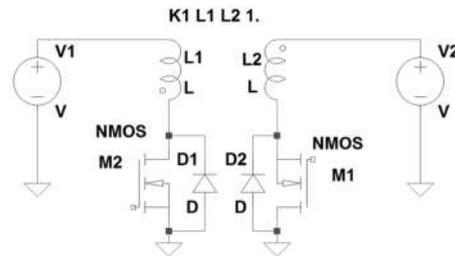
Figure 3. Dual Flyback Power Stage of Bi-directional Converter
